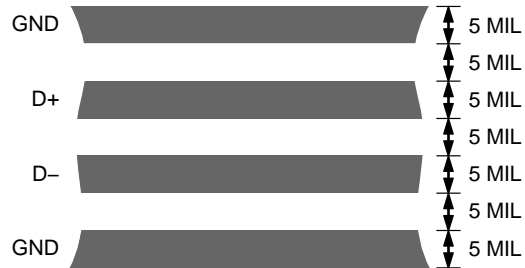
Figure 34. Typical Arrangement of Signal Tracks
