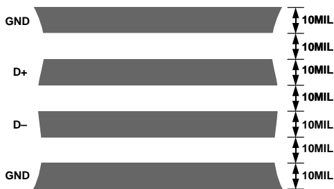
Figure 18. Arrangement of Signal Tracks
