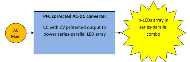
Figure 1. Single Stage Integrated LED Driver (Type 1)
