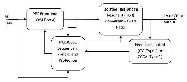
Figure 4. Simplified Control Scheme Offered by NCL30051
