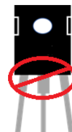
Figure 3. Sideways Bending May Cause Damage
