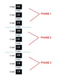
Figure 7. Example Layout for a 1 × 2 MOSFET Combination with a 3 mm Spacing
