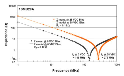
Figure 3. Impedance Characteristic of the 1SMB28A Unidirectional TVS Diode
