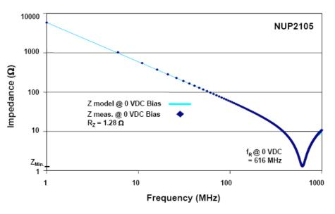
Figure 4. Impedance Characteristic of the NUP2105 Bidirectional TVS Diode
