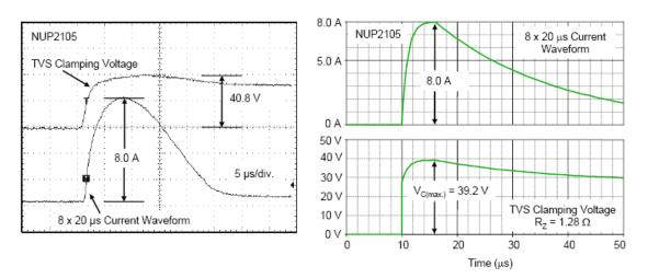
Figure 7. SPICE Predicts a Maximum Clamping Voltage of 39.2 V. The Bench Test Measured Value is 40.8 V
