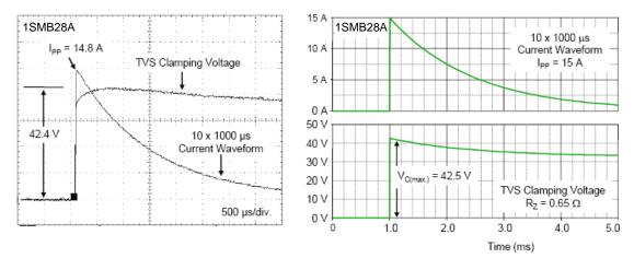
Figure 6. SPICE Predicts a Maximum Clamping Voltage of 42.5 V if R<sub>Z</sub> is equal to 0.65  $\Omega$ . The Bench Test Value is 42.4 V
