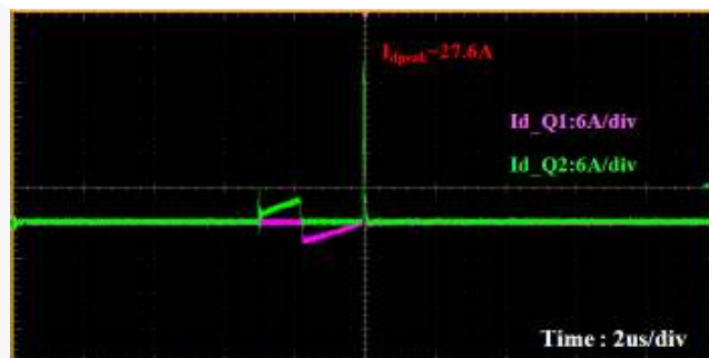
Figure 14. Waveform of Competitor A During Startup
