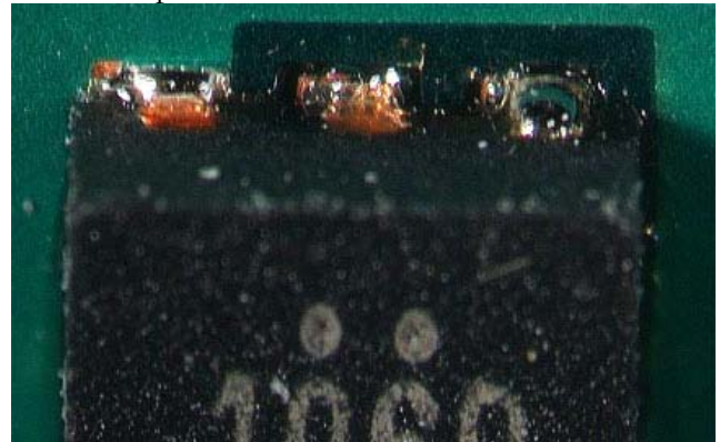
Figure 2: Exposed copper on package edge, with solder wetting after reflow, from singulation process.
