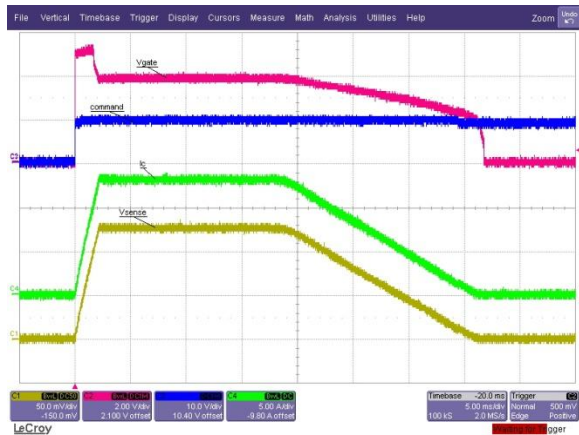
Figure 15. Soft Shutdown (SSD) Waveforms
