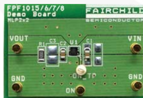
Figure 9. FPF1018 Evaluation Board
