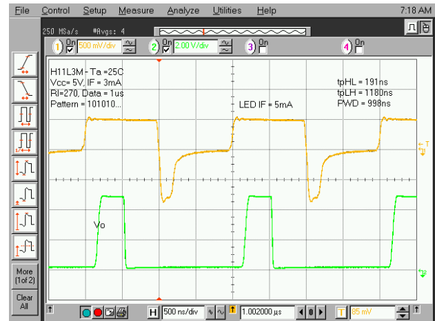
Figure 3. Switching Performance with Peak LED Current at 5 mA
