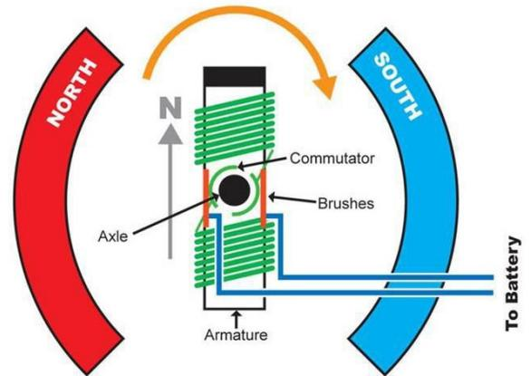
Figure 1 Schematic of a brushed motor
