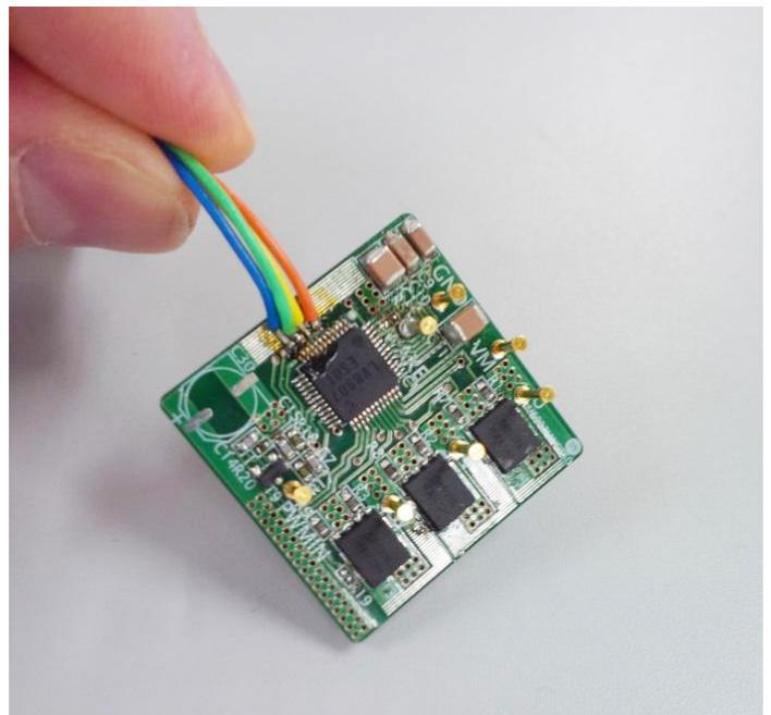
**Figure 2** This brushless motor solution featuring an integrated controller/driver plus three dual FETs.
