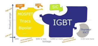
Figure 1. Power Switch Environment [1]
