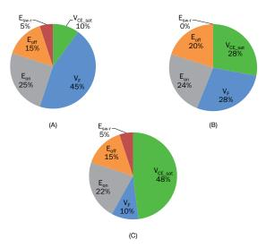
Figure 36. Losses Distribution of a Given IGBT Operating in the Vienna Topology, Half-bridge and Full-bridge
