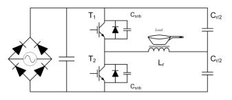
Figure 20. Resonant Half-bridge Topology for Induction Cooking Applications
