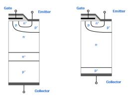
Figure 5. Left) Punch-through (PT) IGBT; Right) Non-punch-through (NPT) IGBT
