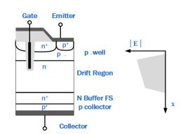
Figure 6. Field Trench Stop IGBT Structure
