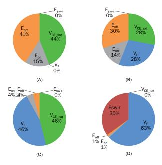
Figure 37. Losses Distribution of a Given IGBT Operating in a T–Type Inverter in the Outer ( $T_1$  and  $T_4$ ) and Inner ( $T_2$  and  $T_3$ ) Position in Inverter and Rectifier Mode
