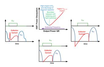
Figure 24. QR Operation Mode Left) Light Load; Center) Mid Load; Right) Heavy Load. Top) IGBT Losses for Different Load Conditions
