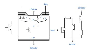
Figure 4. IGBT with Parasitic Structure
