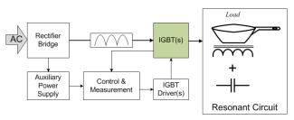
Figure 19. System Block Diagram of Welding Machines
