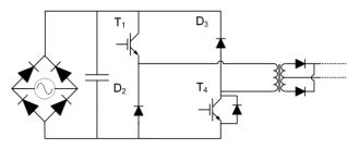
Figure 15. Double Switches Forward Topology
