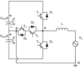
Figure 32. T–Type Converter
