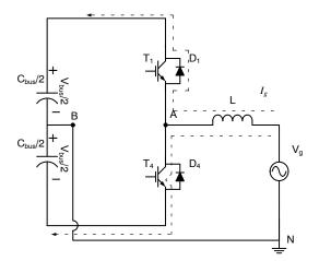
Figure 26. Half-bridge – Operating Waveforms for Negative Current Output
