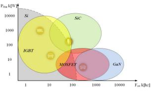
Figure 2. Range of Operation of Silicon and Wide Band Gap Devices
