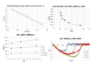
Figure 9. Examples of IGBT and Antiparallel Diode Possible Trade Off
