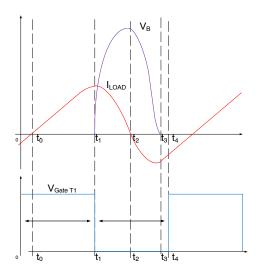
**Figure 23. QR Single – End Inverter and its Associated Waveforms** (Upper graph: current into the resonant coil *L*<sub>r</sub> appears in the red curve while the voltage across *T*<sub>1</sub> is the purple curve.
