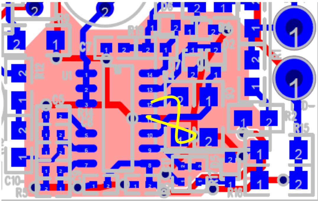
Notice the tight current loop formed by the current sense resistor R4. Pin 11 and Pin 12 are adjacent to make this a naturally tight current loop.
