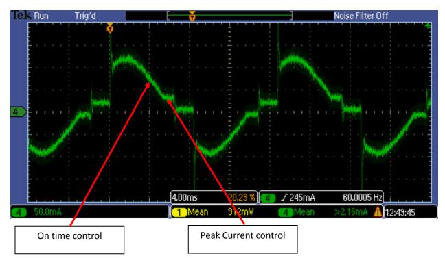
Typical Input Current during Dimming Figure 5.
