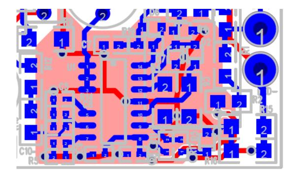
One of the first things to notice is the ground plane under the control circuit (colored in pink). The controller ground pin is pin 11. It is immediately connected to the ground plane through a via.
