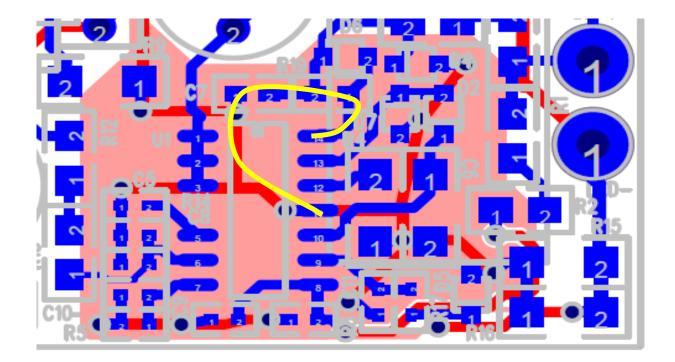
Here the loop for the gate of the HV FET is show in yellow. The gate resistor (R19) is right next to pin 14 which is the gate of the HV FET. The gate capacitor (C7) is directed connector to R19 and the ground plane.
