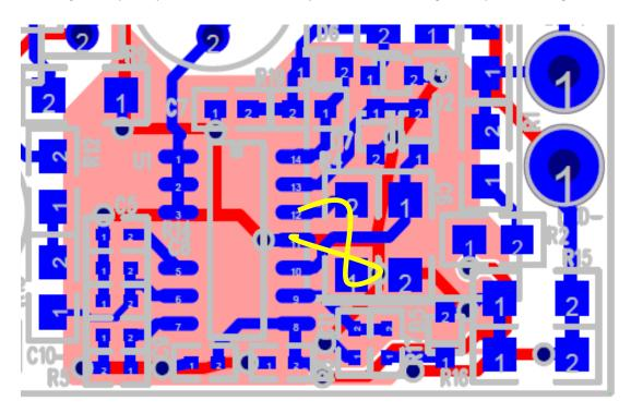
Notice the tight current loop formed by the current sense resistor R4. Pin 11 and Pin 12 are adjacent to make this a naturally tight current loop.
