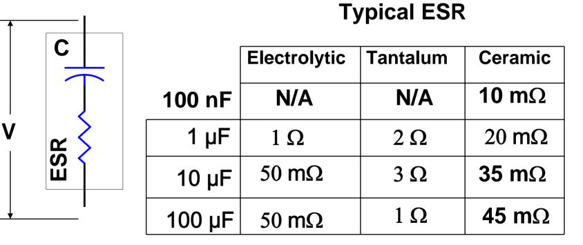
Realistic Capacitor Value on the PCB
