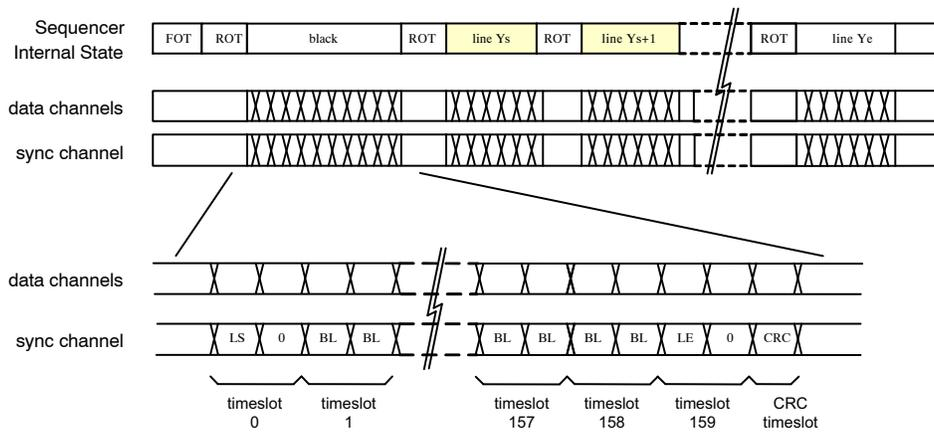
**Figure 19. M1-SM: Time Line for Black Line Readout**
