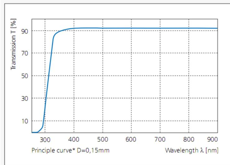
Figure 36. Transmission Characteristics of the Glass Lid
