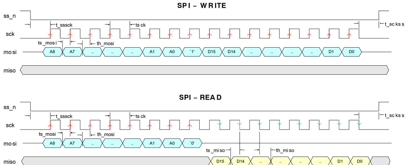
Figure 11. SPI Read and Write Timing Diagram
