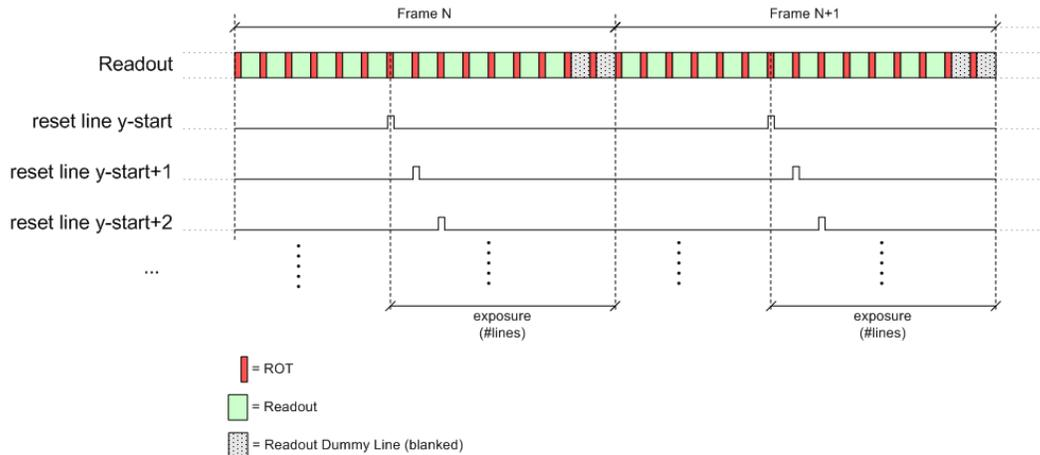
**Figure 12. Integration Control in Rolling Shutter Mode**
