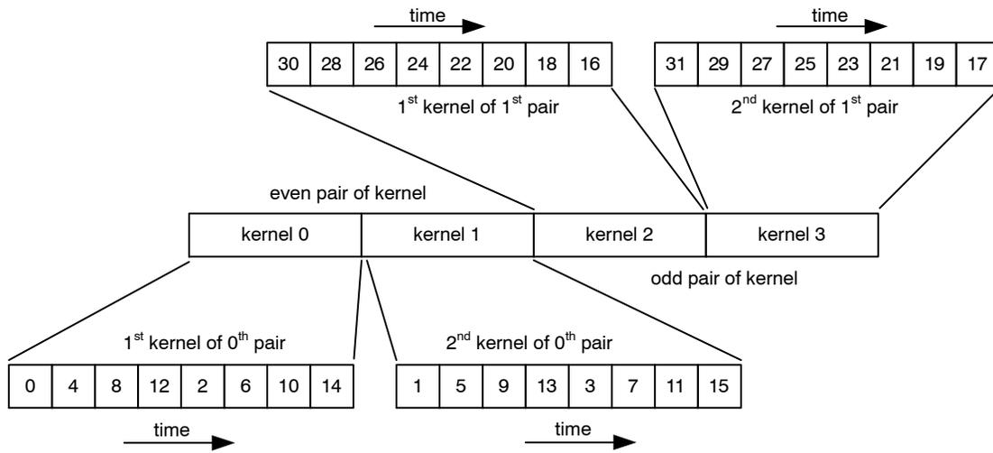
**Figure 30. M2-SM: Data Output Order without Subsampling**
