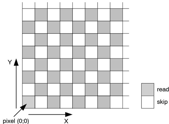
**Figure 16. Checkerboard Subsampling**
