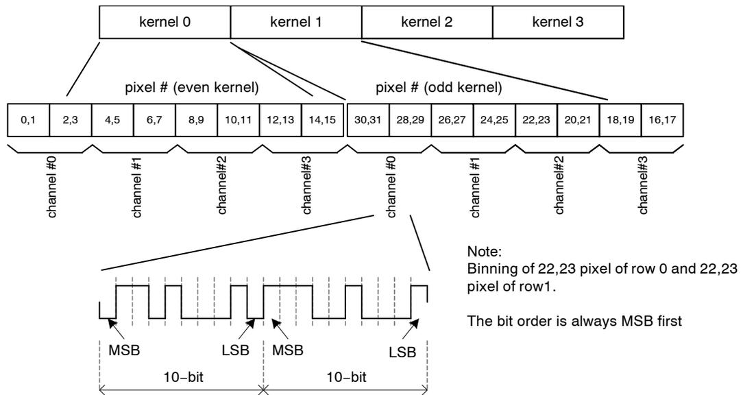
**Figure 27. M1-SM: Data Output Order for 2 x 2 Binning**
