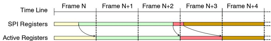
**Figure 9. Frame Synchronization of Configurations (no freezing)**
