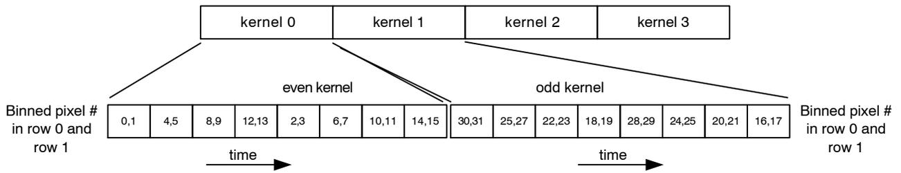
**Figure 33. M2-SM: Data Output Order for 2 x 2 Binning**
