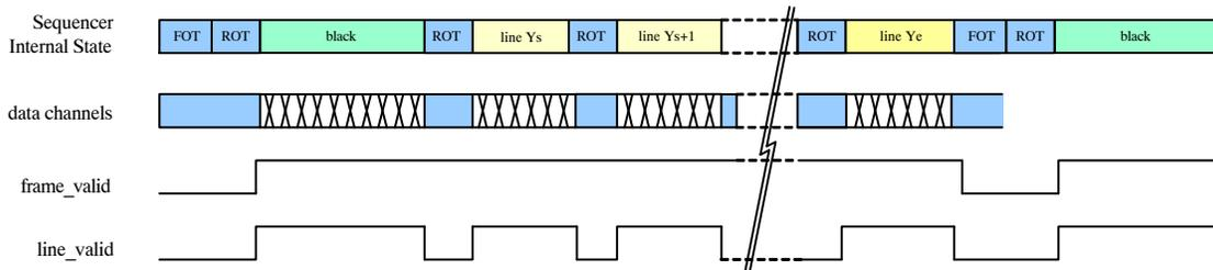
**Figure 28. M2–SM: Frame Timing Indication**
