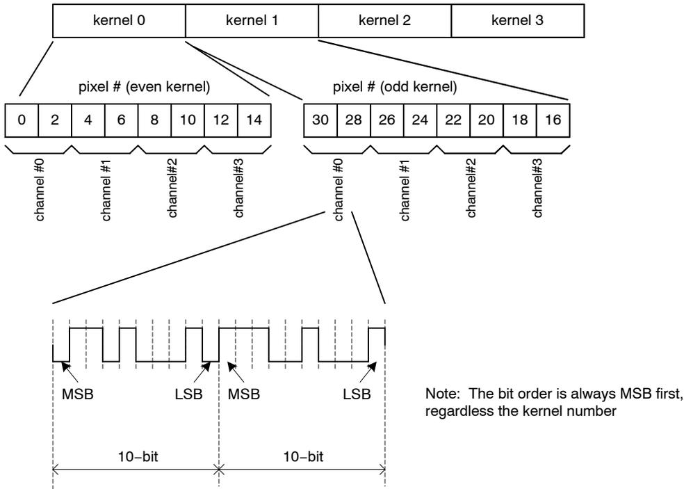
**Figure 24. M1-SM: Data Output Order for Read-1-Skip-1 Subsampling**
