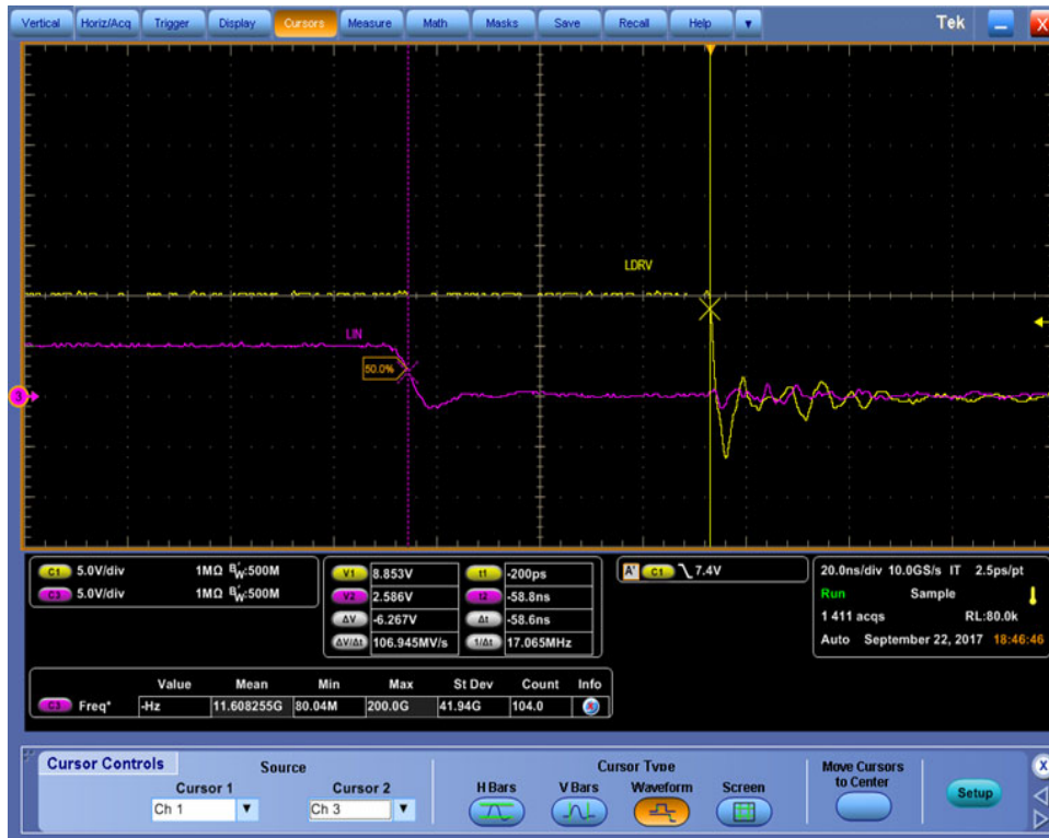
Figure 30. Low Side Turn-Off Propagation Delay (NCP51530A)
