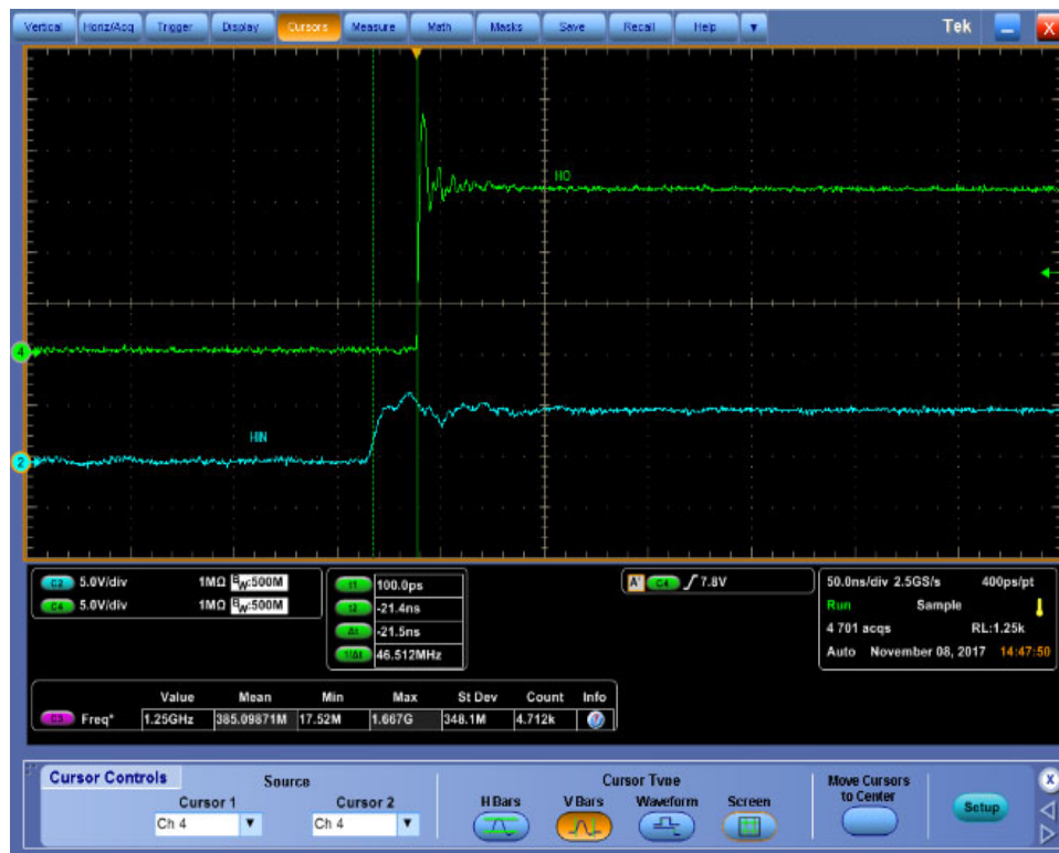
Figure 31. High Side Turn-Off Propagation Delay (NCP51530B)
