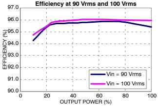
Figure 4. Efficiency at 90 Vrms and 100 Vrms
