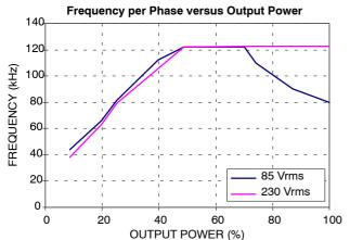
Figure 7. Switching Frequency per Phase versus
