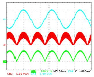
Figure 8. Input Voltage and Current at 90 Vrms
