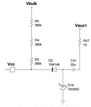
Figure 1. Optional Startup Circuit
