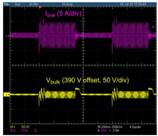
Figure 14. Transient Load Response at 115 Vrms (from 20% to 100% of P<sub>out,max</sub>)
