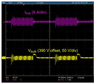
Figure 15. Transient load response at 230 Vrms (from 20% to 100% of P<sub>out,max</sub>)
