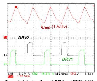
Figure 11. Inductors Current, DRV1 and DRV2 at 230 Vrms
