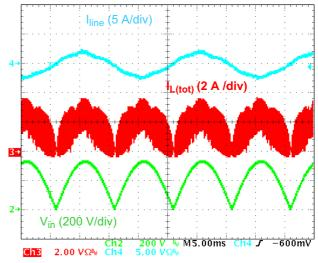
Figure 9. Input Voltage and Current at 230 Vrms
