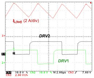
Figure 10. Inductors Current, DRV1 and DRV2 at 90 Vrms
