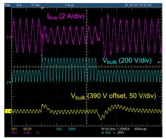
Figure 13. Line Transient at half the output load
