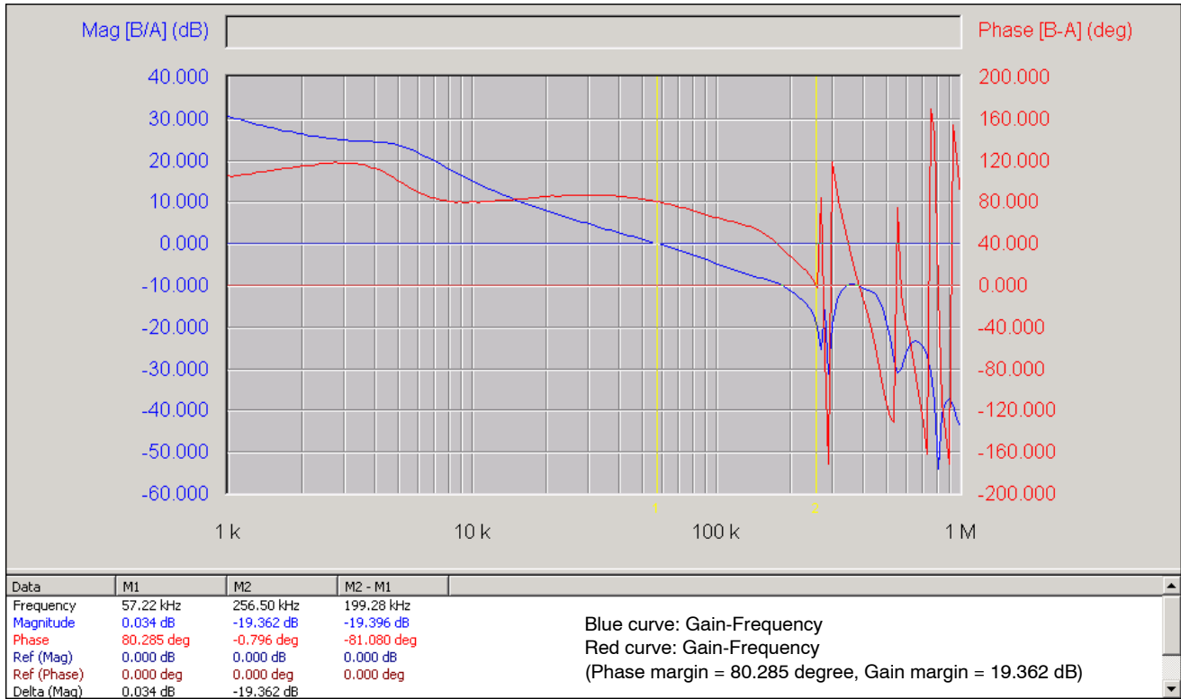
Figure 14. Closed-loop Voltage Loop-gain of the NCP1587
