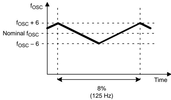
Figure 30. Frequency Jittering
