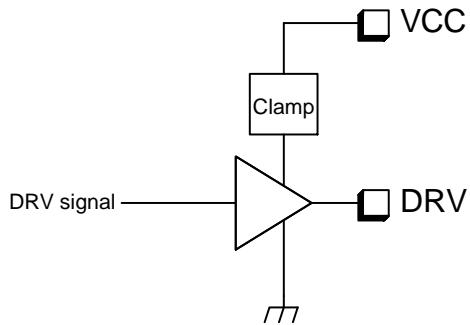
Figure 31. Clamped Driver
