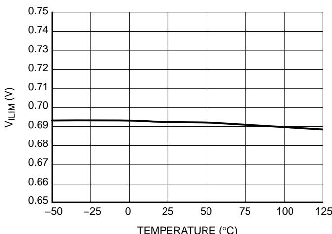
Figure 5. Maximum Internal Current Setpoint
