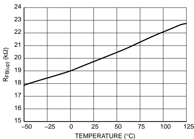
Figure 9. FB Pin Internal Pull-up Resistor
