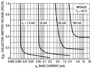
Figure 9. Collector Saturation Region
