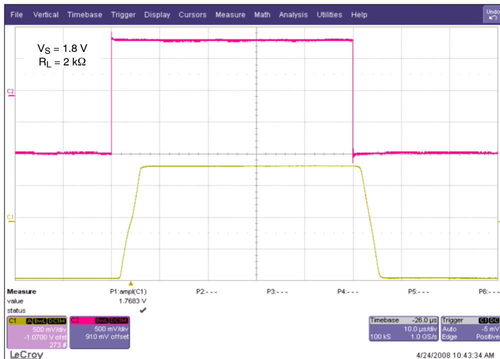
Figure 18. Small Signal Noninverting Response
