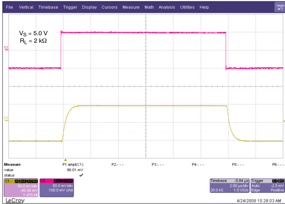
Figure 18. Small Signal Noninverting Response
