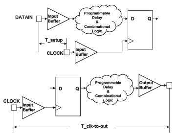
Figure 7. Definitions of Setup and Clock-to-Out Time
