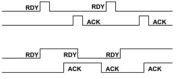
Figure 24. Strobe and Toggle Waveforms
