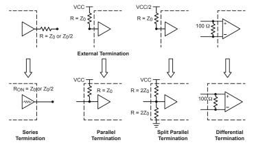
Figure 19. On-Chip Digital Controlled Impedance
