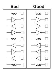
Figure 18. Group the Input Pads and the Output Pads and Isolate them with Pwr/Gnd
