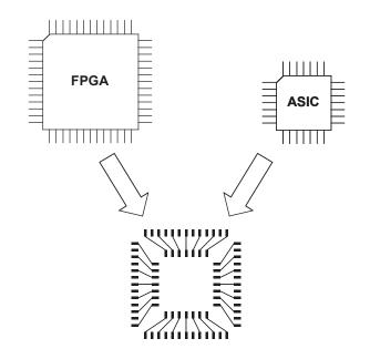
Figure 2. Package Shrink and Concentric Pad Rings
