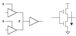
Figure 31. Floating Internal Tri-State Bus
