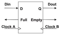
Figure 25. Passing Data Between Clock Domains with a FIFO
