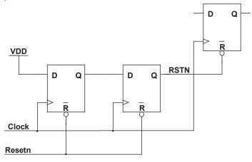
Figure 17. Synchronized Reset Circuit
