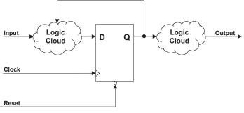
Figure 21. Synchronous Design
