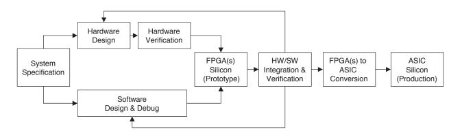
Figure 3. FPGA-to-ASIC Conversion Methodology
