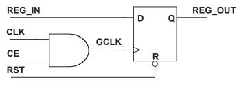
Figure 26. Gated Clock Schematic
