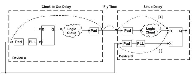
Figure 5. System Timing Diagram
