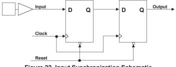
Figure 22. Input Synchronization Schematic
