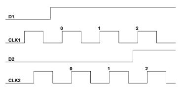
Figure 11. Multi-Cycle Timing
