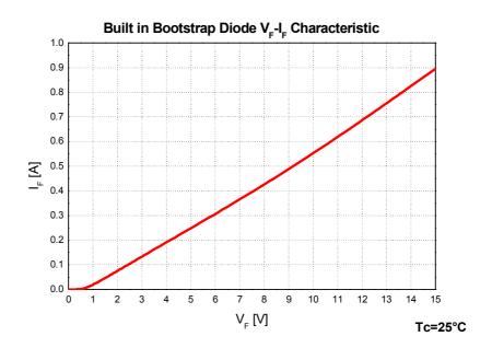
Figure 2. Built in Bootstrap Diode Characteristics(typ.)
