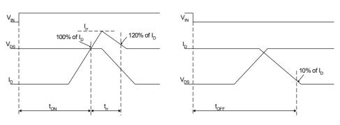
(a) Turn-on (b) Turn-off Figure 6. Switching Time Definition
