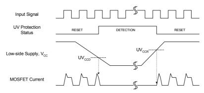
Figure 8. Undervoltage Protection (Low-side)
