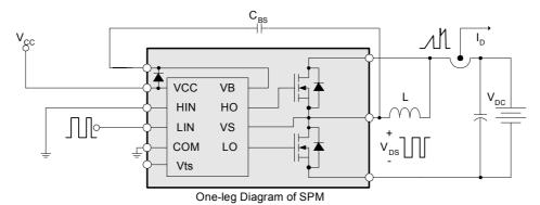
Figure 7. Switching and RBSOA(Single-pulse) Test Circuit (Low-side)
