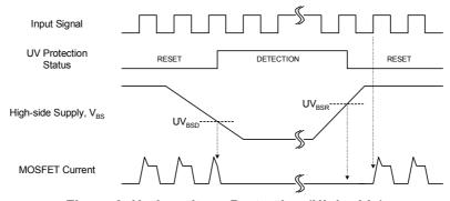
Figure 9. Undervoltage Protection (High-side)
