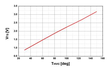
Figure 5. Temperature profile of Vts(typ.)
