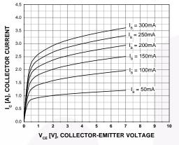
Figure 1. Static Characteristic
