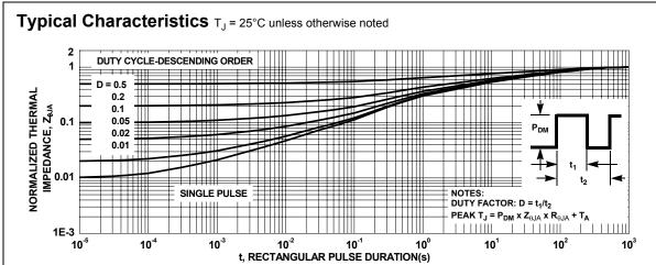
Figure 13. Transient Thermal Response Curve
