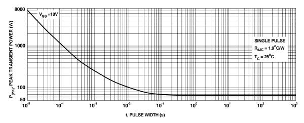
Figure 13. Single Pulse Maximum Power Dissipation
