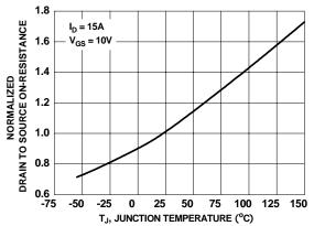
Figure 3. Normalized On-Resistance vs Junction Temperature
