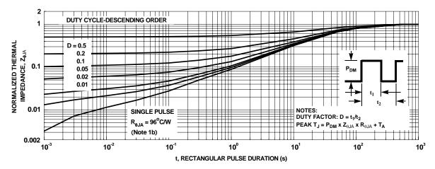
Figure 16. Transient Thermal Response Curve
