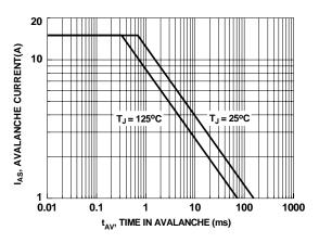
Figure 9. Unclamped Inductive Switching Capability
