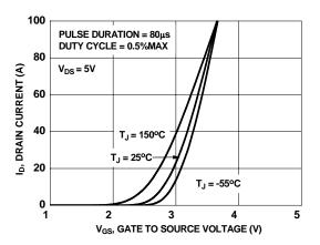
Figure 5. Transfer Characteristics
