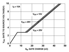
Figure 7. Gate Charge Characteristics
