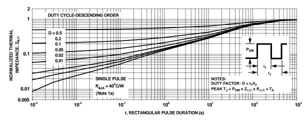
Figure 15. Transient Thermal Response Curve
