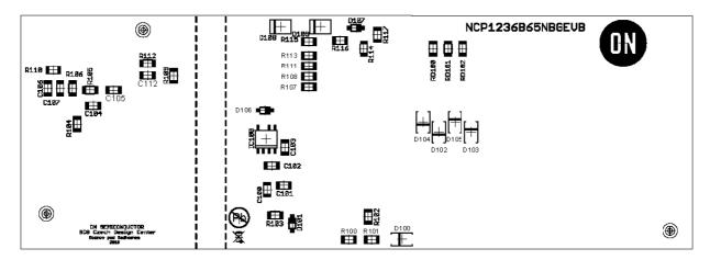
Figure 28. Component Placement on the Bottom Side (Bottom View)
