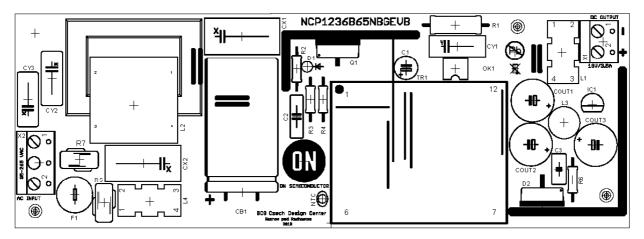
Figure 27. Component Placement on the Top Side (Top View)
