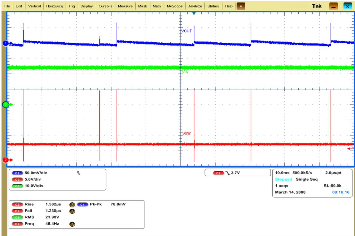
Figure 11- NCP3063 Output Ripple at 24 V to 5 V at a no load
