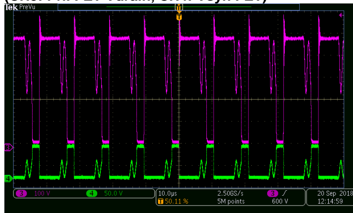
90 Vac input, 20V4.5A output (CH3: Pri. FET Vdrain, CH4: Vsyn FET)
