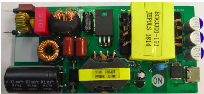
Figure 1, Overall cycle of 90 W TYPE-C PD Adapter Solution
