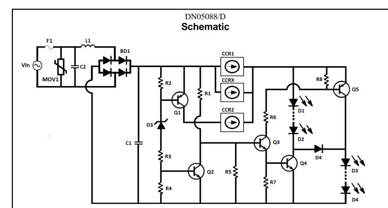
Figure 2 – Two-Stage Parallel-to-Series LED Lighting Circuit, with Switch-In CCR. It is possible to mount for an inductor (L1) and an additional capacitor on the board for additional EMI filtering, but generally these are not needed and L1 has a 0 ohm resistor in its place on the evaluation board. C2 may also be populated to ensure compatibility with a small minority of dimmers which require bleeding current even when manually switched off.
