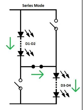
Figure 3 – The LED configuration is dynamically adjusted by the control circuitry. When AC instantaneous voltage is relatively low, the LEDs are configured in parallel. At relatively high AC instantaneous voltages the LEDs run in series.
