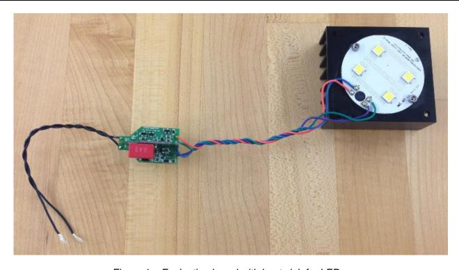
Figure 1 – Evaluation board with heat sink for LEDs.
