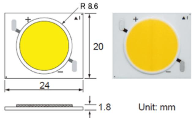
The Sharp GW5D series (image above) is rated at typically 2300-2600 lumens at 25 °C case temperature when driven at 700 mA and the forward voltage range is 34-40 V dc under those conditions.
