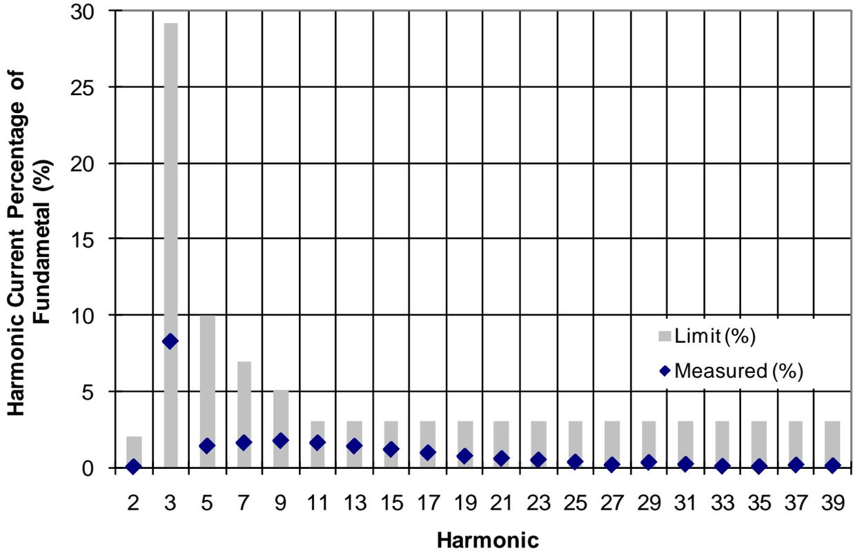
**Figure 2: EN61000-3-2 Class C Input Current Harmonic Test**
