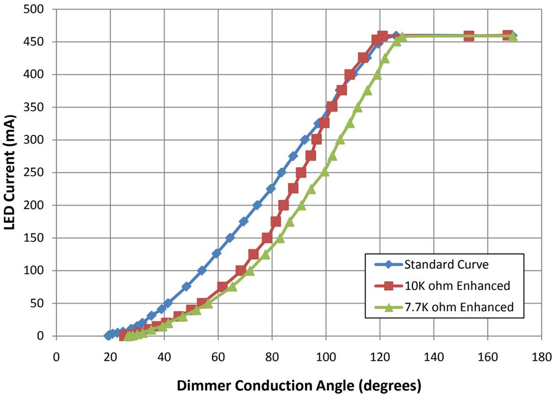
Figure 3: 230 Vac Dimming Characteristics (Rin = 300 kΩ)
