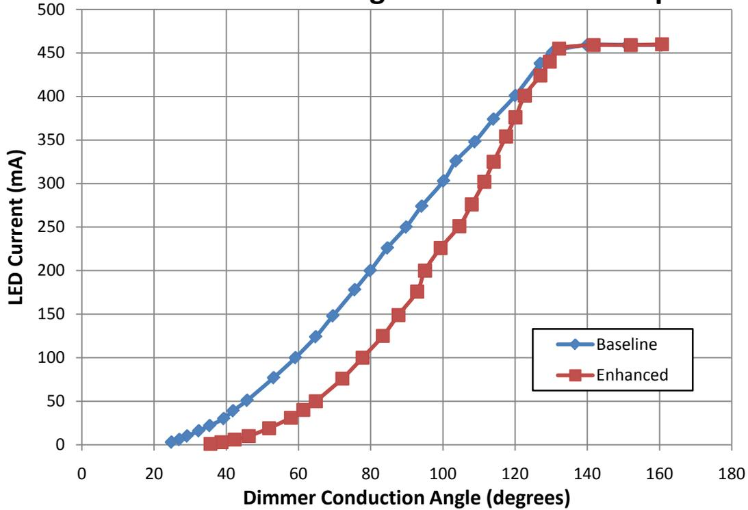
Figure 2: 115 Vac Dimming Characteristics (Rin = 150 kΩ)
