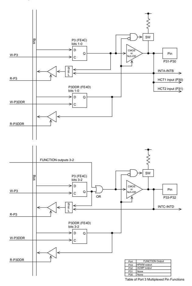
Port 3 Block Diagram Option: Output type (CMOS or Nch-OD) selectable on a bit basis.
