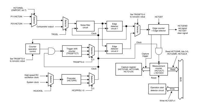
Figure 3.8.1 High-speed Pulse Width/Period Measurement Counter 2 Block Diagram
