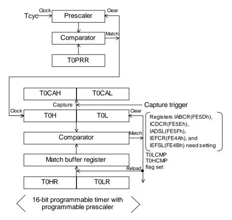
Figure 3.3.3 Mode 2 Block Diagram (T0LONG = 1, T0LEXT = 0)
