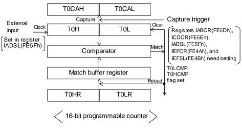
Figure 3.3.4 Mode 3 Block Diagram (T0LONG = 1, T0LEXT = 1)
