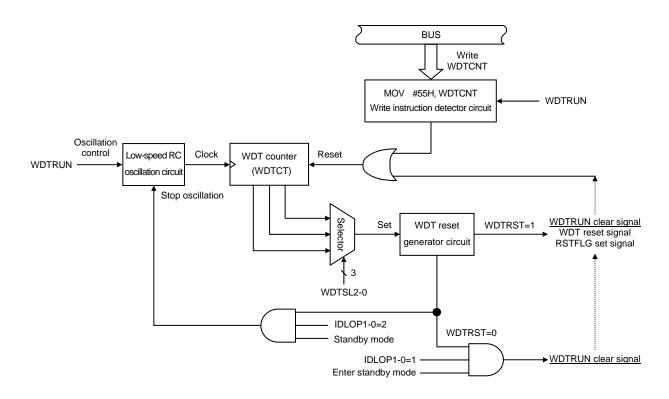
Figure 4.6.1 Watchdog Timer Operation Block Diagram
