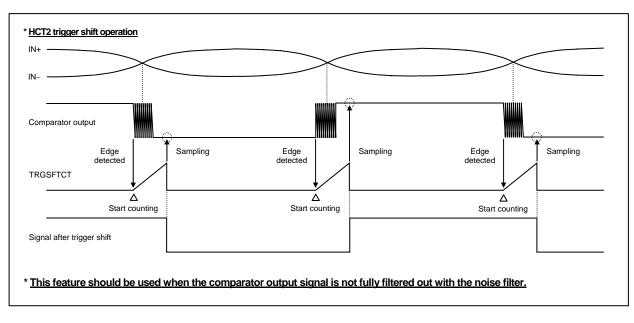
Figure 3.8.3 Sample Input Trigger Signal Shift Operation Waveforms (TRGSFT2 to TRGSFT0 set to a nonzero value)
