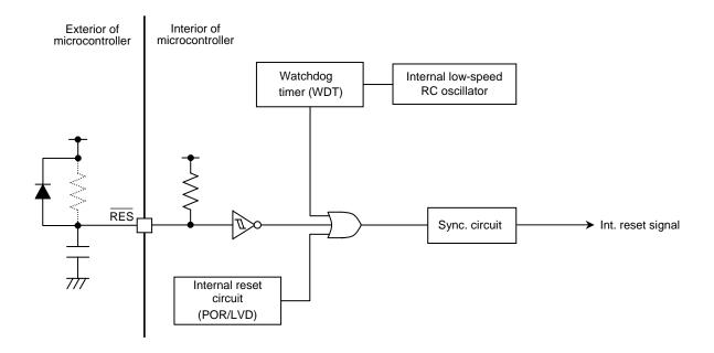
Figure 4.4.1 Sample Reset Circuit Block Diagram
