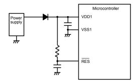
Figure 4.5.4 Example of Power Interruption / Voltage Fluctuation Countermeasures
