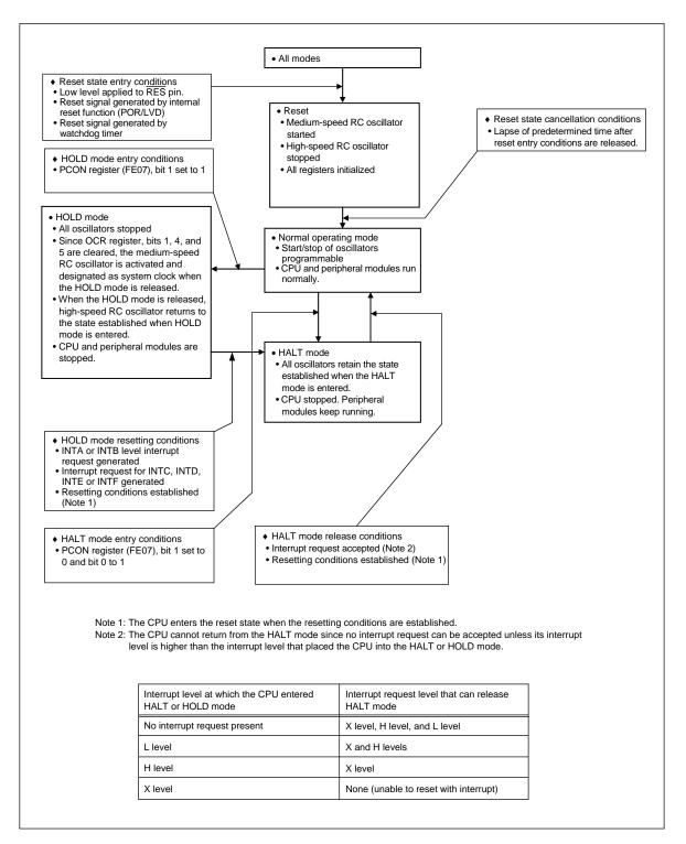
Figure 4.3.1 Standby Mode State Transition Diagram
