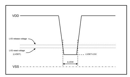
Figure 4.5.3 Example of Power Interruption or Voltage Fluctuation Waveform
