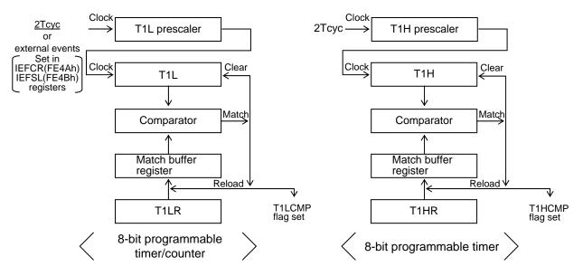
Figure 3.4.1 Mode 0 (T1LONG = 0) Block Diagram
