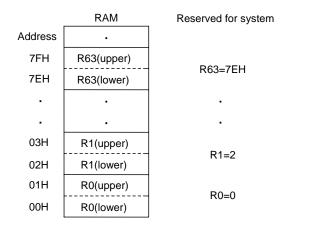
Fig. 2.10.1 Allocation of Indirect Registers
