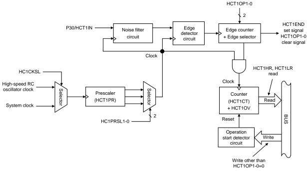
Figure 3.7.1 High-speed Pulse Width/Period Measurement Counter 1 Block Diagram
