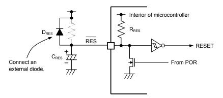
Figure 4.5.7 Sample External POR Circuit Configuration
