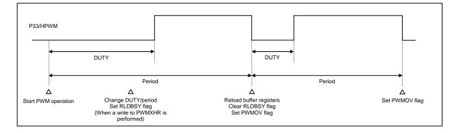
Figure 3.6.2 Sample Continuous Output Mode Waveform (PWMINV=0)
