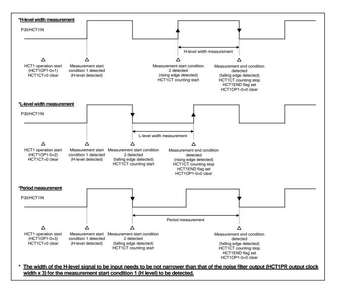
Figure 3.7.2 Sample High-speed Pulse Width/Period Measurement Counter 1 Waveforms
