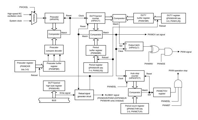
Figure 3.6.1 High-speed 12-bit PWM Block Diagram
