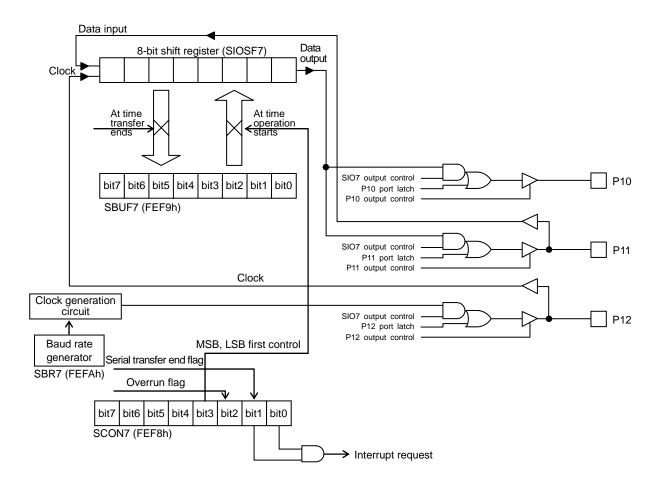
Figure 3.5.1 SIO7 Synchronous 8-bit Serial I/O Block Diagram
