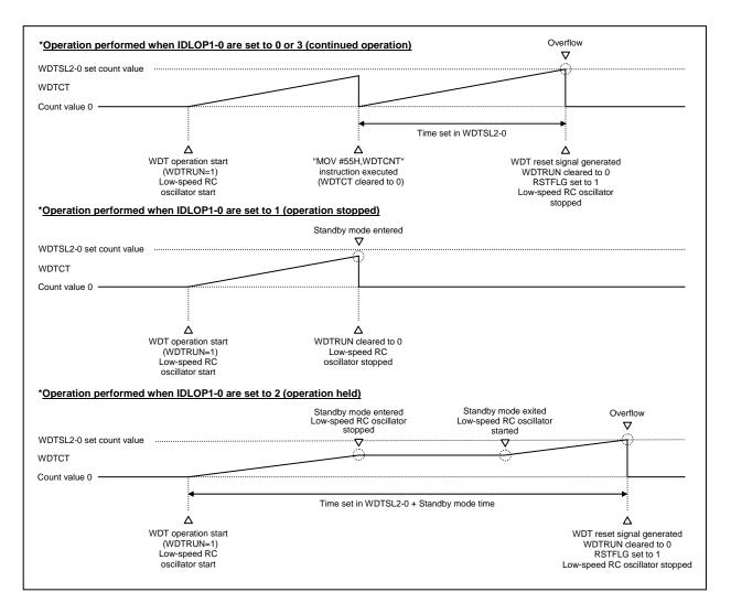
Figure 4.6.2 Sample Watchdog Timer Operation Waveforms
