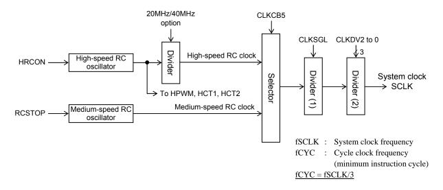
Figure 4.2.1 System Clock Generator Block Diagram
