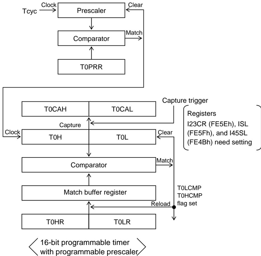
Figure 3.3.3 Mode 2 Block Diagram (T0LONG = 1, T0LEXT = 0)
