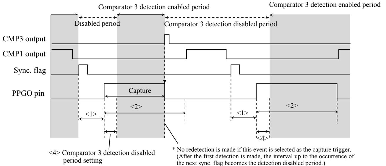
**Figure 3.10.9 PPG Output Timing 4**
