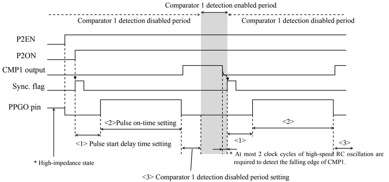
**Figure 3.10.6 PPG Output Timing 1**
