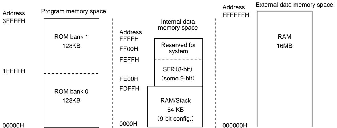
*Note: SFR is the area in which special function registers such as the accumulator are allocated (see Appendix A-I).*
