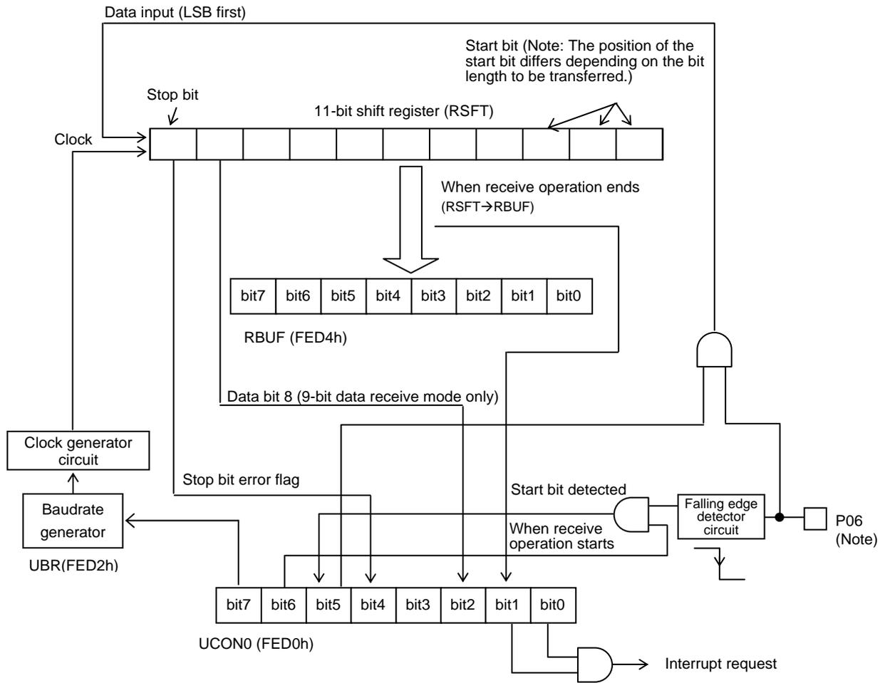
*Note: Bit 6 of P0DDR (at FE41) must be set to 0 when the UART1 is to be used in receive mode (The UART1 will not function normally if this bit is set to 1).*
