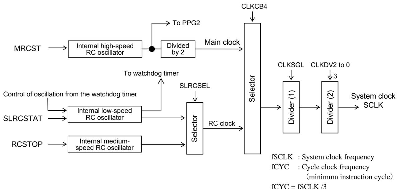
Figure 4.2.1 System Clock Generator Circuit Block Diagram
