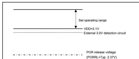
*Note 5: The operation guarantee values (voltage/operating frequency) shown in the examples vary with the microcontroller type. Be sure to refer to the latest "SANYO Semiconductors Data Sheet" and select the proper setting level .*
