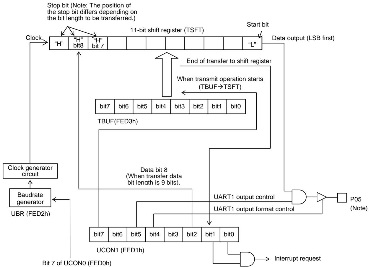
Note: Bit 5 of P0DDR (at FE41) must be set to 0 when the UART1 transmit data is to be output (Transmit data is not output if this bit is set to 1).
