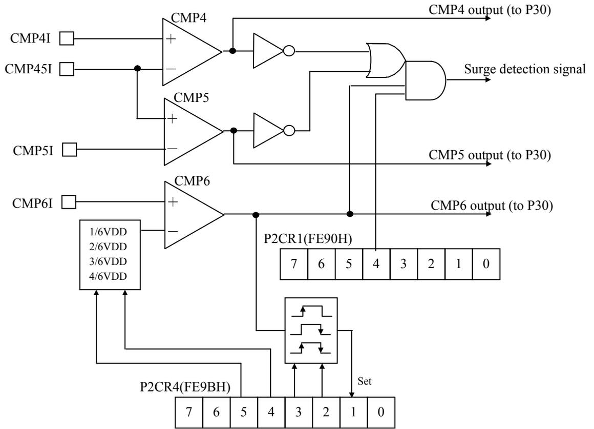
Figure 3.10.2 Surge Detector Circuit Block Diagram
