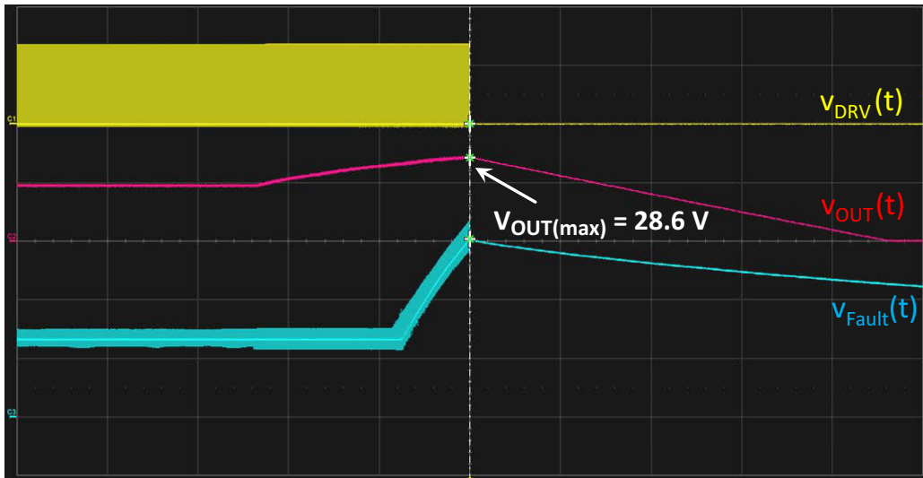
Figure 10. OVP Event on Fault Pin
