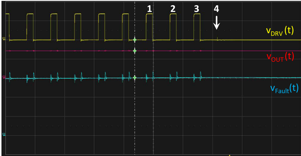
Figure 9. 4 Consecutives Pulses to Validate the OVP Fault
