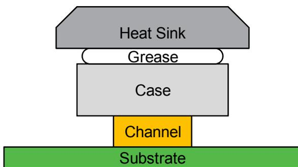
$$R_{\theta JA} = R_{\theta JC} + R_{\theta GR} + R_{\theta HS}$$
