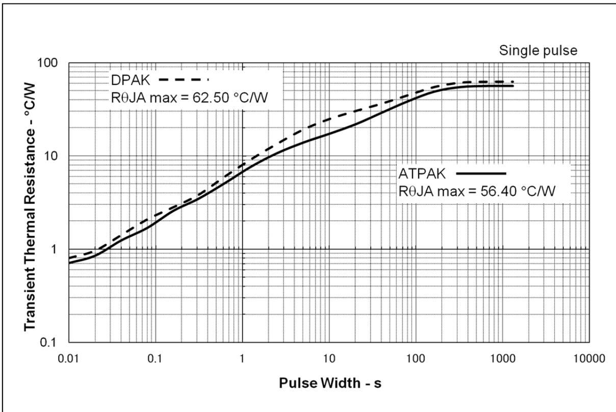
Figure 6 Transient Thermal Resistance with Heat Sink
