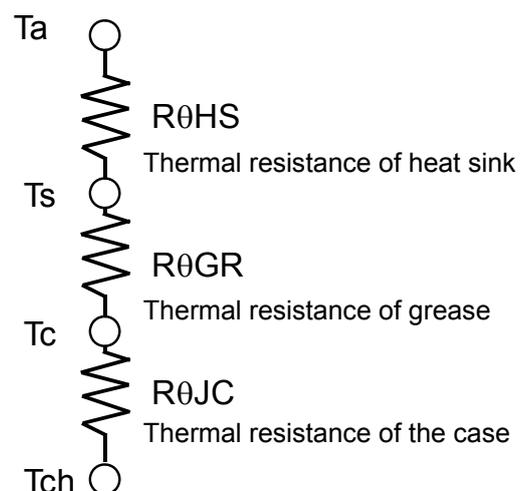
Figure 1. Thermal Resistance Model
