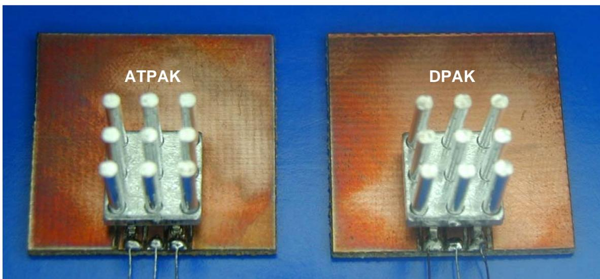
Figure 4. Actual Evaluation Board with Heat Sink
