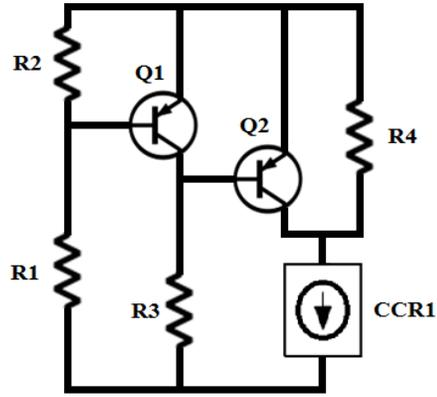
Figure 7. PNP-Based Schematic of a High-Voltage Protection Block
