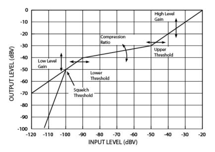
Figure 2. Independent Channel I/O Curve Flexibility
