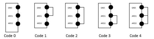
Figure 6. Wiring Diagrams for Automatic Receiver Detection
