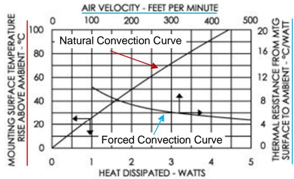
**Figure 3. Example Manufacturer Data Sheet Thermal Performance Graph**
