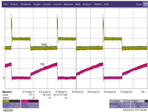
Figure 8. Boost Coil Current Waveform For V_{in} = 24 \text{ V} - 10\% , V_{out} = 125 \text{ V} , P_{out} = 73 \text{ W}
