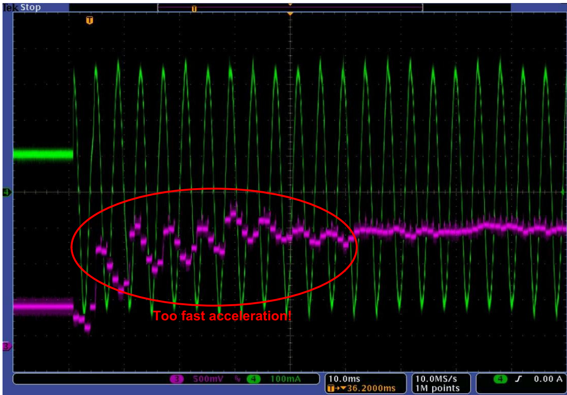
Figure 34. Too Fast Acceleration Results in Overshoots
