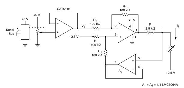
Figure 12. Programmable Current Source/Sink
