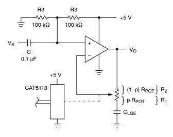
Figure 2. Programmable Voltage Amplifier
