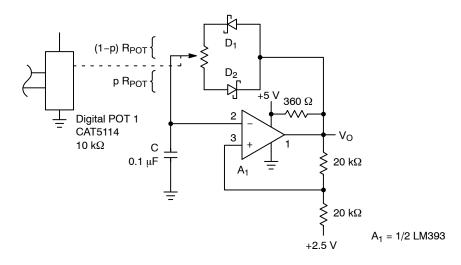
Figure 9. Programmable Duty Cycle
