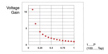
Figure 3. Gain versus Wiper Setting
