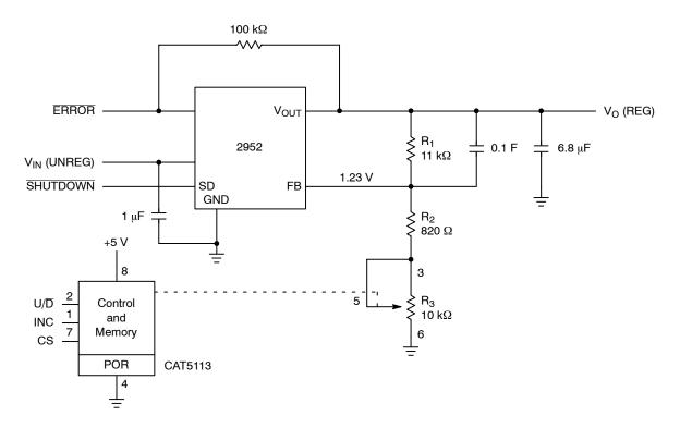
Figure 11. Programmable Voltage Regulator
