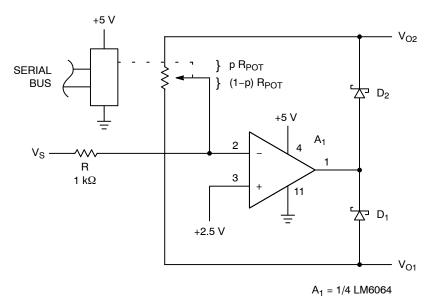
Figure 5. Dual Gain Amplifier
