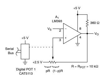
Figure 13. Programmable Schmitt Trigger
