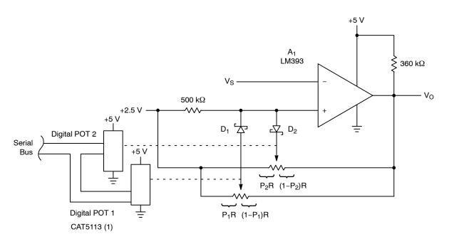
Figure 15. Schmitt Trigger with Independently Programmable Limits
