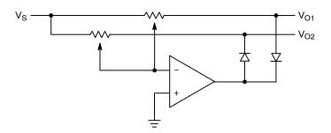
Figure 7. Dual Independent Gain Amplifier
