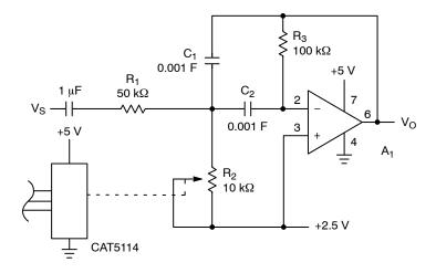
Figure 10. Programmable Bandpass Filter
