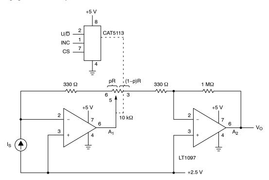
Figure 16. Programmable I to V Convertor
