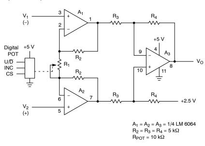
Figure 4. Programmable Instrumentation Amplifier
