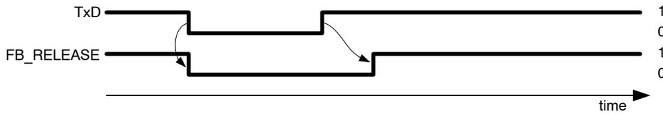
**Figure 4. Function of a Feedback Suppression Block (FBS)**
