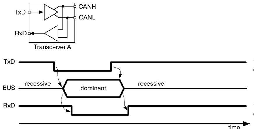
Figure 1. Simplified Model and Timing of a High-speed CAN Transceiver
