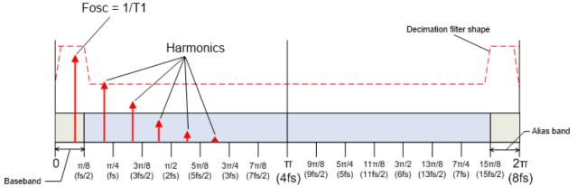
Figure 2. Slow ADC Output Oscillation
