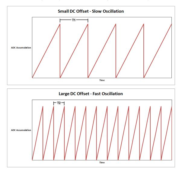
Figure 1. Period of ADC Output Oscillation
