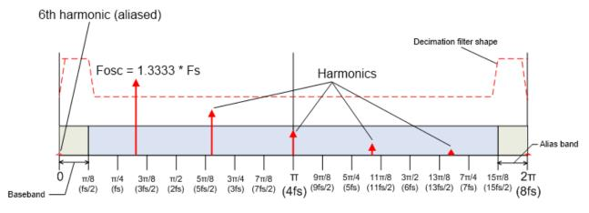
Figure 4. Ideal ADC Output Oscillation
