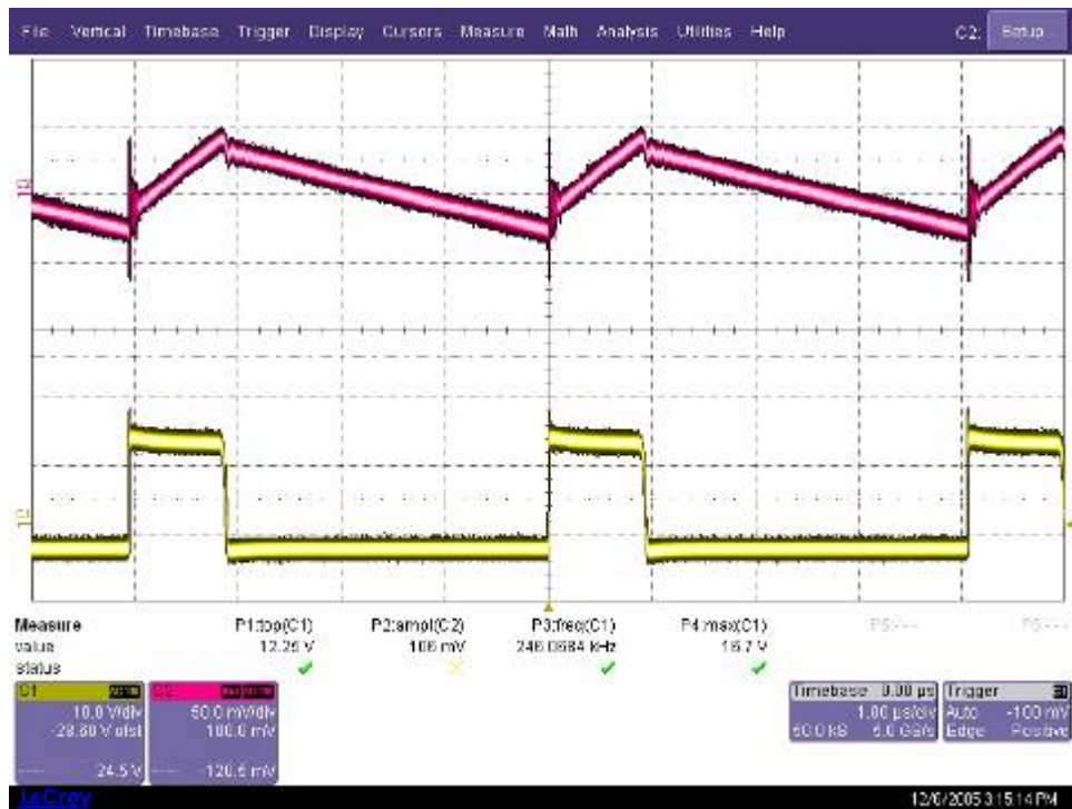
Figure 19. Vin = 18 V, Vout = 3.3 V, Iout = 1.5 A, C1 = Vout, C2 = VSW
