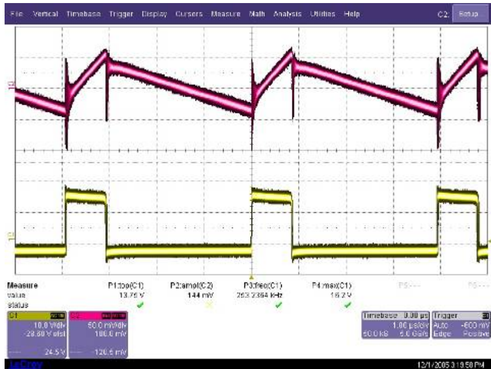
Figure 11. V_{in} = 18\text{ V} , V_{out} = 3.3\text{ V} , I_{out} = 1.5\text{ A} , C1 = V_{out} , C2 = V_{SW}
