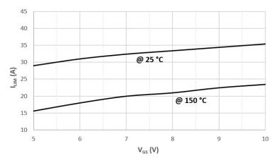
a) Measured current limit across gate-source voltage in NCV8401
