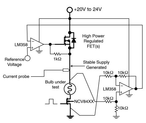
Figure 19. Idealized Circuit to measure the Inrush Profile of a Bulb against a known Driver
