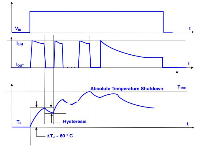
Figure 10. Idealized Wave-set depicting DTSD Protection (not drawn to scale)
