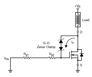
Figure 15. Inductive Switching Circuit Diagram
