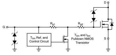
**Figure 4. Simplified Input Circuit**
