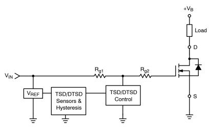
Figure 8. Simplified Over-temperature Shutdown Circuit
