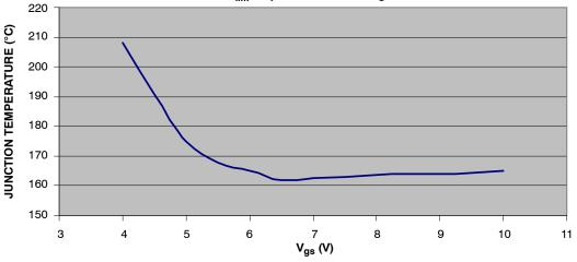
Figure 12. Typical Temperature Limit Shutdown as a Function of Gate Voltage
