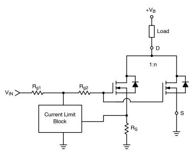
Figure 5. Simplified Current Limit Circuit
