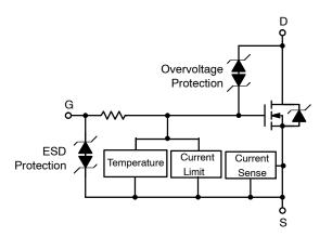
Figure 2. Generic Block Architecture of Low Side SmartFETs
