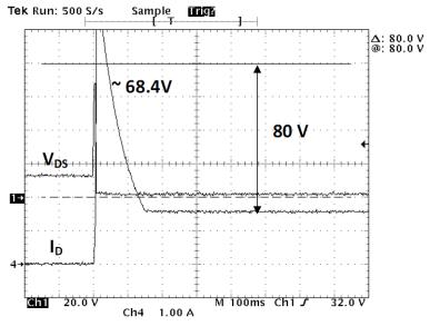
b) Fail:  $V_{GS}$  = 0 V, Va + Vs = 75 V (Device clamps at 68.4 V)
