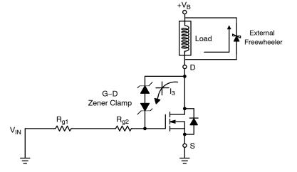
Figure 17. Application Example with External Diode for Inductive Flyback
