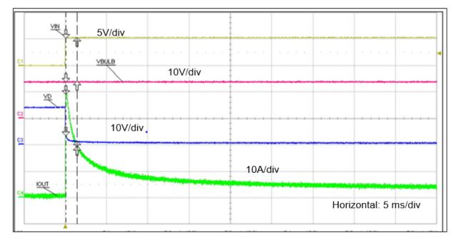
Figure 18. Inrush Profile of 4\*R10W when Switched On at -40°C
