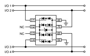
In the case of applications in which a positive supply reference is not available or full isolation is required, the internal TVS could be used as the reference, so for this purpose, pins 2 and 3 are not connected. In this case, the steering diodes will conduct whenever the voltage on the protected line exceeds the working voltage of the TVS plus one diode drop ( $Vc = Vf + V_{TVS}$ ).
