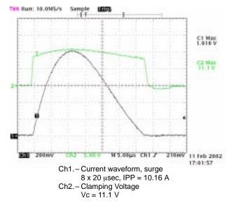
NOTE: The pulse current was measured with a current monitor with conversion factor of 100 mV = 1.0 Amp.
