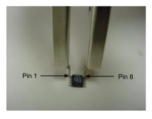
Figure 5. Measurement Between Pins 1 and 8
