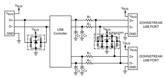
Figure 16. ESD Protection for USB Port
