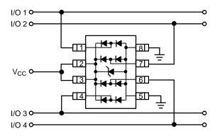
For this configuration, connect pins 2 and 3 directly to the positive supply rail (Vcc), the data lines are referenced to the
