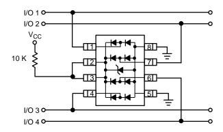
The NUP4201DR2 can be isolated from the power supply by connecting a series resistor between pins 2 and 3 and Vcc. A resistor of 10 Kohms is recommended for isolation purposes. The internal TVS and steering diodes remain biased, which provides the advantage of lower capacitance.
