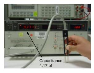
Figure 4. Capacitance Measurement Between I/O Lines
