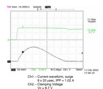
NOTE: The pulse current was measured with a current monitor with conversion factor of 100 mV = 1.0 Amp.
