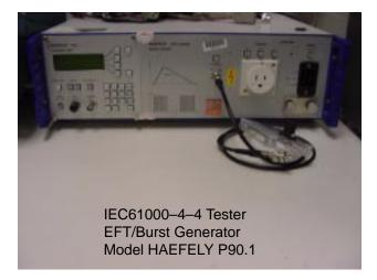
Figure 12. EFT Generator
