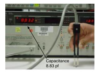
Figure 6. Capacitance Measurement Between I/O Lines and Ground
