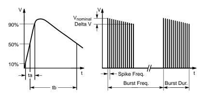
Figure 11. EFT Tester's Technical Characteristics
