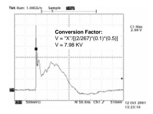
Figure 10. Real Waveform Sample Taken from ESD Generator
