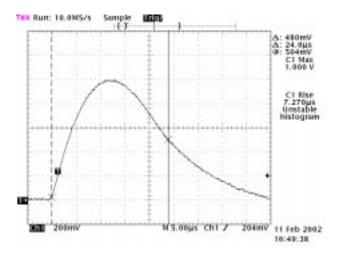
Figure 13. Double Exponential Pulse 8 x 20  $\mu sec$
