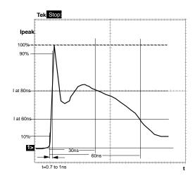
Figure 8. Typical Output's Waveform of the ESD Generator
