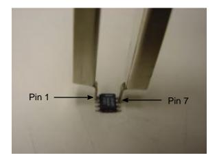
Figure 3. Measurement Between Pins 1 and 7
