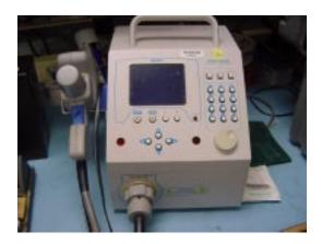
Figure 9. ESD Generator, NoiseKen ESS-2000
