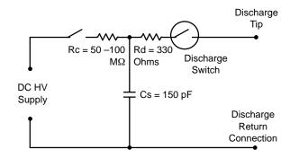
Figure 7. ESD Generator, Simplified Diagram
