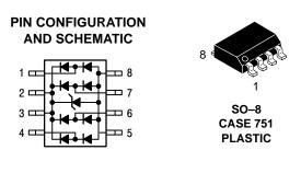
Figure 1. NUP4201DR2 Device's Schematic
