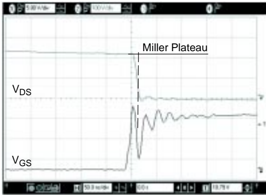
Figure 25. A small glitch occurs at the Miller transition
